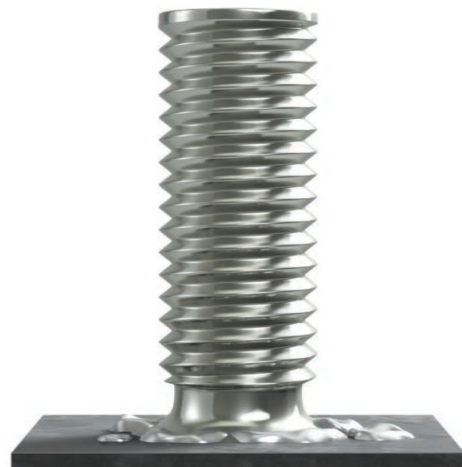
f. Stud weld made with excessive heat
