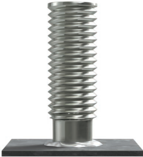
a. Good stud weld with a good flash formation
