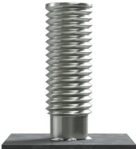
e. Stud weld made with insufficient heat
