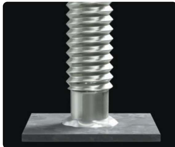
d. Gun is withdrawn from the welded stud, and ferrule is removed.
