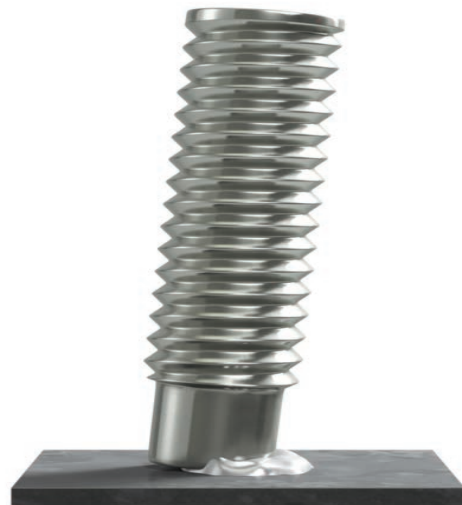
d. Poor alignment
