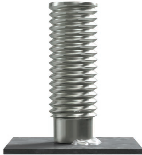
b. Stud weld in which plunge is too short
