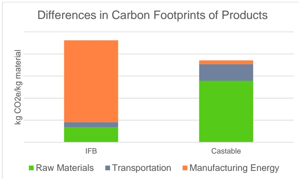
Figure 9: Typical Difference in Carbon Footprints of Common Refractory Products
