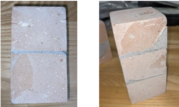
Figure 11 – Mortar joint compression at room temperature
