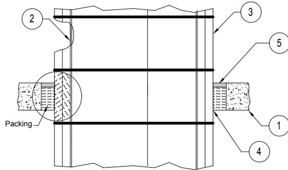
XL Insulation continuous through rated floor/ceiling assembly
